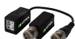
VT-TR4K Passive Video Balun Transmitter / Receiver Pair for HD-TVI / AHD / CVI for Distances up to 1440'
