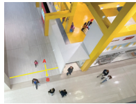
LINE CROSSING Track People or Vehicles as Entering or Exiting Designated Areas
