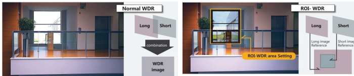
ROI (Region of Interest) WDR achieves superior exposure compensation specifically in exact areas of interest while reducing HDD storage space.
