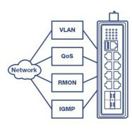
L2+ Management Provides an easy to use web management interface for traffic management controls such as VLAN, QoS, access controls, link aggregation, troubleshooting, SNMP monitoring, and per port MAC restriction.
