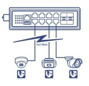
**PoE Power** A 240W PoE power budget supplies up to eight Power over Ethernet devices, and includes advanced PoE port controls such as enabling / disabling PoE, power priority, PD alive check, and power scheduling.
