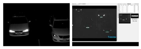
Clear Image Captured with IR Illuminators and Headlight Filter
