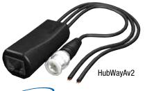
HubWayAv2 Video Balun/Combiners are compatible with all HubWay and HubSat UTP Transceiver Hubs. They allow for video and data transmission and power over CAT-5 or higher structured cable to AC or DC fixed cameras or PTZs.
