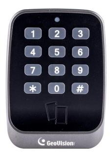
GV-RKV1355 is a vandal-resistant keypad reader capable of reading PIN codes and access cards. To successfully resist vandalism, the reader's case is made of zinc alloy, making it suited for high-security locations such as banks and prisons. Featured with Wiegand and RS-485 interfaces, GV-RKV1355 can be integrated to any standard access control systems. Furthermore, the reader complies with IP66 ingress protection, making it perfect for both indoor and outdoor applications.
