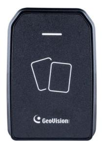
The card reader GV-R1355, which has Wiegand and RS-485 interfaces, can be integrated into any standard access control system.
