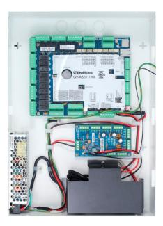
GV-AS8111 Kit is a cabinet containing a GV-AS8111, a power adapter board, a power supply and a casing for backup battery. The power supply provides power to GV-AS8111 Kit and up to 8 output devices (12V, 0.5A per device).
