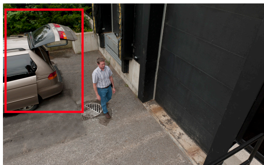
The "Loitering Detection" analytic triggers an alarm when a person or object lingers in a particular area for too long.
